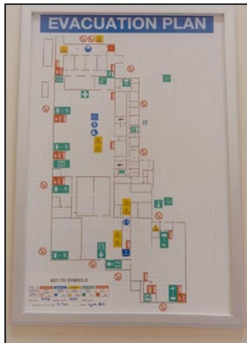
**Figure 74** Evacuation plan showing assembly points and isolation points for utilities
