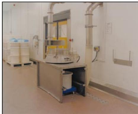
**Figure 12** Dust extraction on sieve unit
