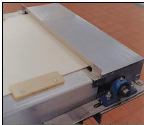
**Figure 52** Fixed guard over in-running nip end roller of conveyor
