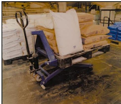
**Figure 25** Adjustable-height, pedestrian-operated pallet truck transporting 25 kg sacks
