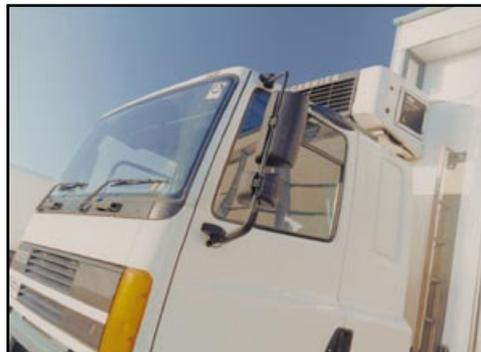
**Figure 36** Delivery vehicle with fixed ladder for maintenance of refrigeration unit (controls are in the cab)
