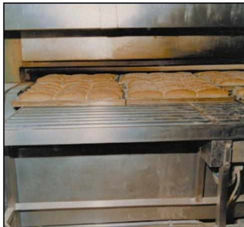
**Figure 2** Bread rolls exiting a tunnel oven
