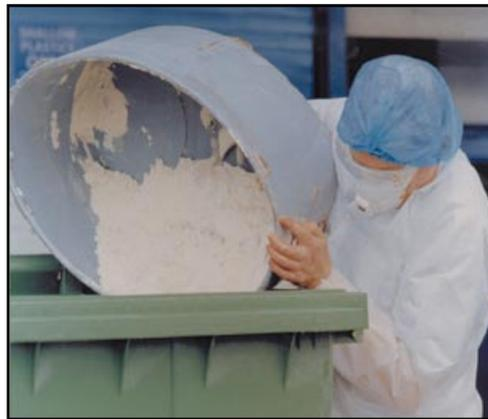
**Figure 20** Use of protective clothing and RPE for emptying vacuum cleaner drum
