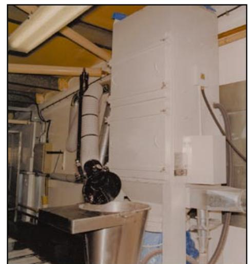
**Figure 13** Dust extraction at sack-tip point
