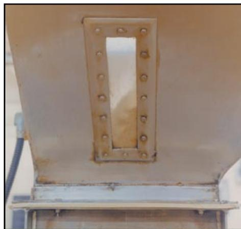
**Figure 53** Vision panel on dough-divider hopper (see Table 8)
