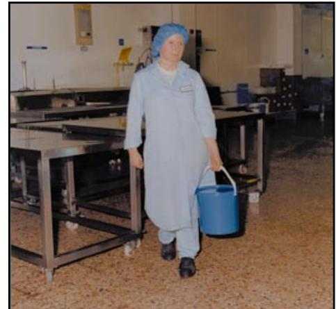
**Figure 30** Lidded container for transporting liquid to avoid spillage and floor contamination
