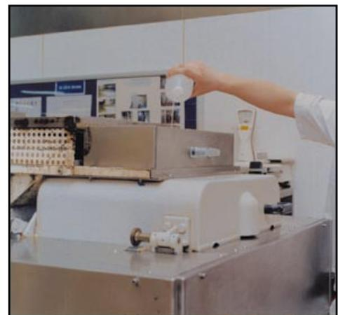
**Figure 54** Dough-divider with sliding-drawer dough feed and use of divider oil to prevent dough sticking
