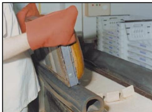
**Figure 56** Rubber knock-out bar on de-panning table
