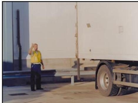
**Figure 34** Banksman in high-visibility waistcoat reversing delivery vehicle
