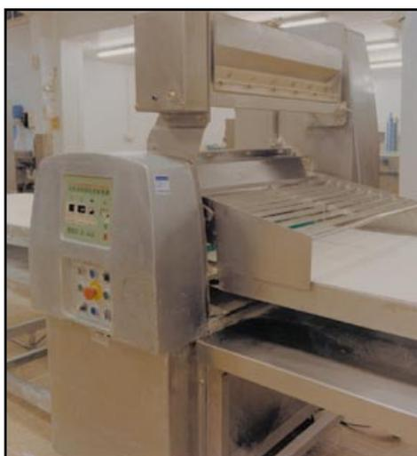
**Figure 47** Dough brake with trip guards
