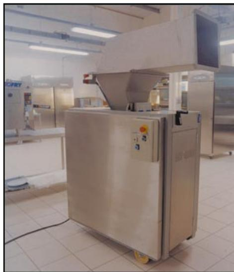
**Figure 49** Dough divider with hinged, interlocked, swan-neck device
