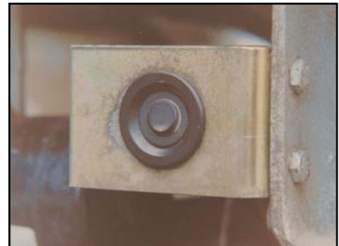
**Figure 35** Ultrasound sensor mounted on rear of vehicle (brakes are automatically applied if the vehicle comes within 1 m of an object)
