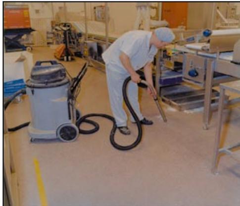
**Figure 16** Use of a vacuum cleaner to clean up flour spillage
