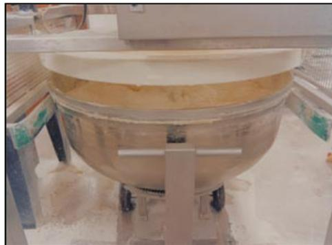
**Figure 14** Hopper outlet incorporating lid which locates over mixing bowl to contain dust
