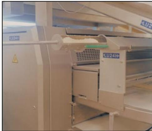
**Figure 15** Removeable, covered flour sprinkler on production line
