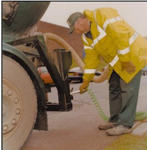
**Figure 64** Connecting earthing cable to flour tanker
