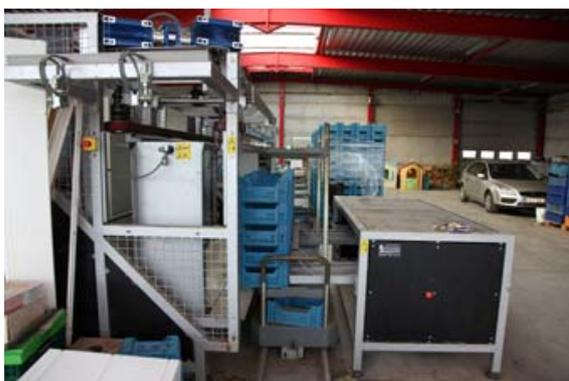
**Picture 6: Conveyor system of the new weighing installation**
