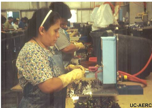
Fig. 3. A worker using a pneumatic shears to cut plant material in nursery propagation.
