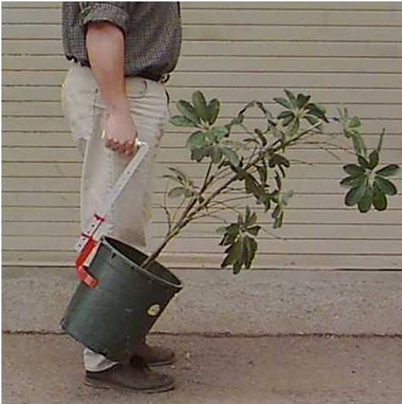
Fig. 2. Adjustable extended handle for handling nursery potted plants.
