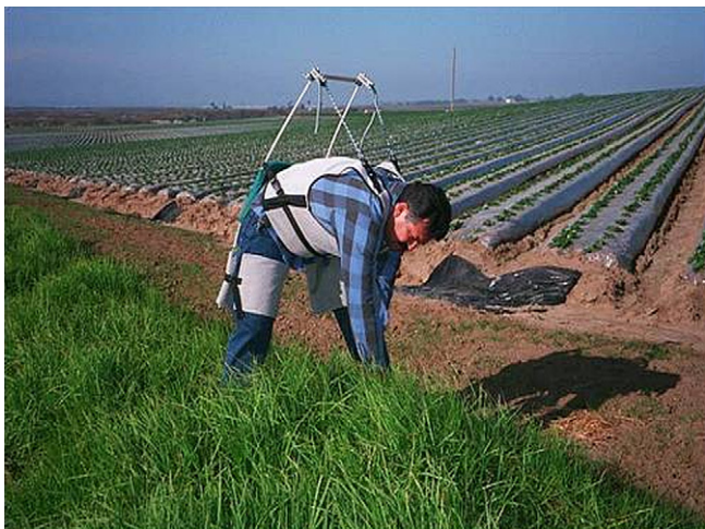
Fig. 8. Personal load transfer device worn by a farm worker (ErgoAg, Aptos, CA).
