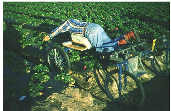
Fig. 7. An example of a prone workstation to control the need for stooping.
