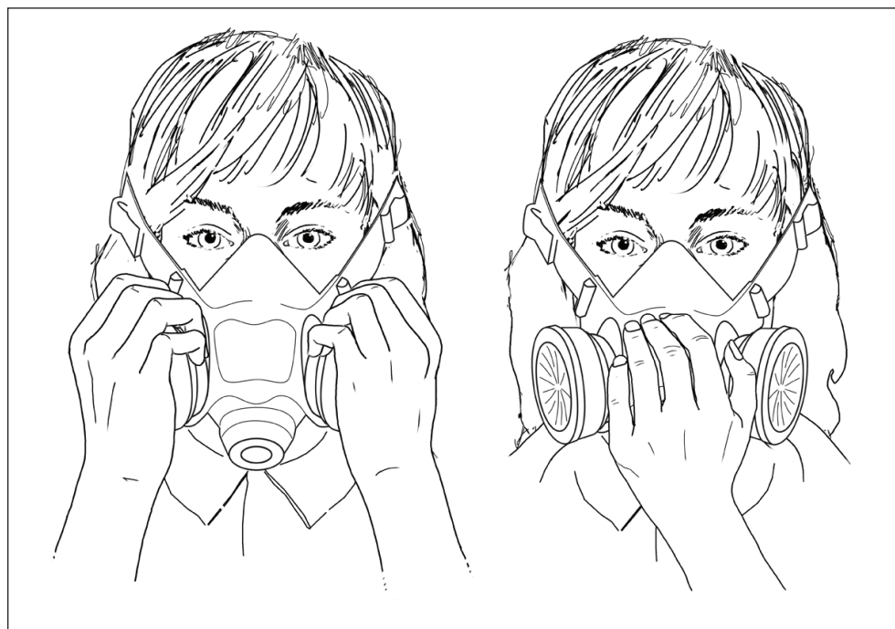
Inhalation check (left) and exhalation check (right) for a half-facepiece respirator
